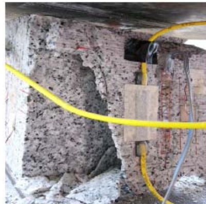
Specimen 2 after failure (Face 1 being sheared off)
